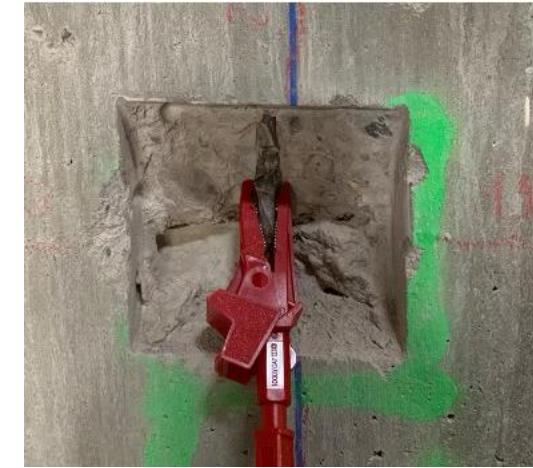
Exposure of steel and connection with an alligator clip
