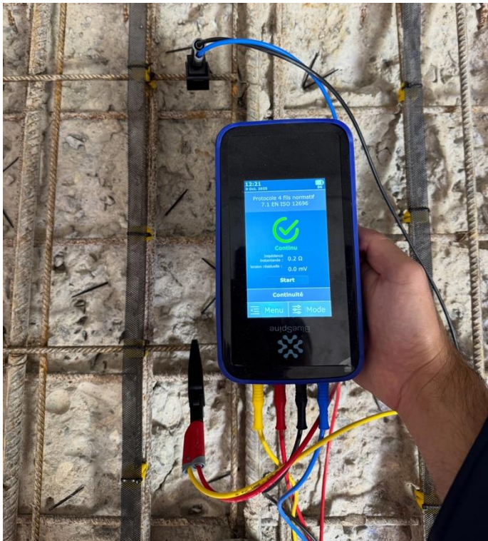
Standard compliant measurement 4 cables (EN ISO 12696) Performed with BlueSpine Q-Box
